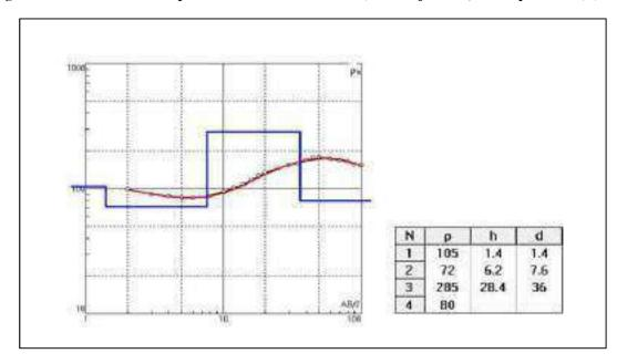
Fig-6.4:VES Curve and interpreted results at Badadhara (Near Resevior, Inside Plant Area) (VES 2)
