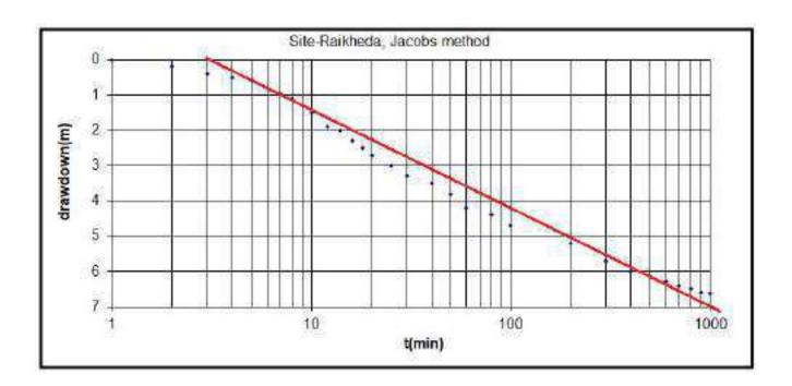
The pumping test data has been analyzed by Jacob's straight line method of the pumping data of the observation well. The calculation is given below.
