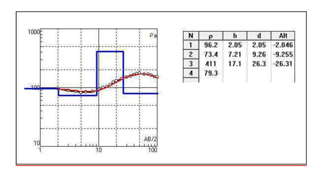
Fig-6.5:VES Curve and interpreted results at Badadhara (Near Coal Yard, Outside of plant area)(VES3)
