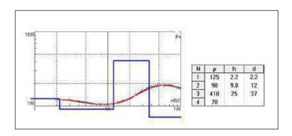
Fig-6.3: VES Curve and interpreted results at Badadhara (Near Urja Road, Inside plant area) (VES 1)
